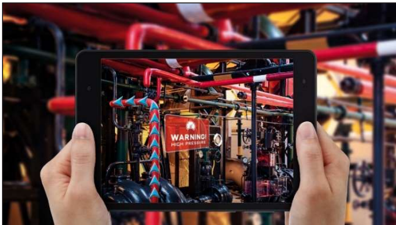
Figure 6: Example of a factory floor scanning application in the form of augmented reality: the additional arrows and warning dialog window appear overlaid on top of the actual system of pipes, valves, and actuators. The user can thus make a quick decision to ensure the continued safe operation of the plant.
