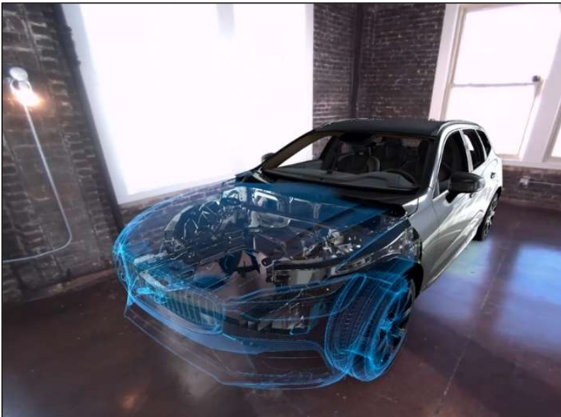
Figure 10: A high-resolution digital twin of a Volvo car model appearing, layer by layer, before the user of the Varjo XR-1 head-mounted display in a real environment. The user can enter the vehicle and get transported into a different location.
