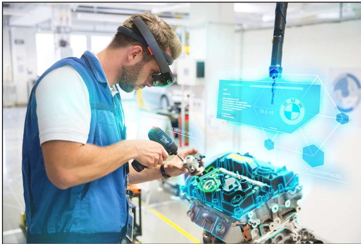
Figure 12: Microsoft HoloLens used in a production process at BMW. The digital twin serves here as a guide for the engineer.
