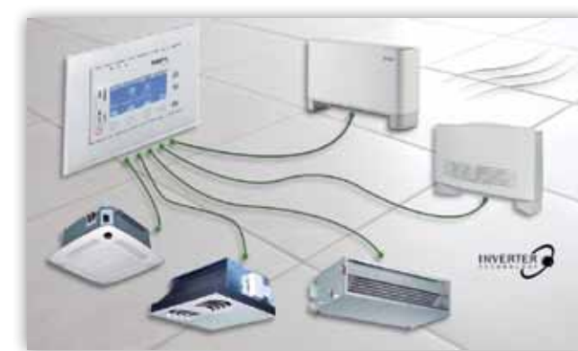
Thanks to inverter technology, the equipment continuously monitors the air volume flow, adjusting it at each instant, to the actual needs of the room to be cooled or heated. This leads to great benefits in all that refers to electricity savings, comfort and a low noise level, as compared with a traditional 3-speed on-off fancoil.
