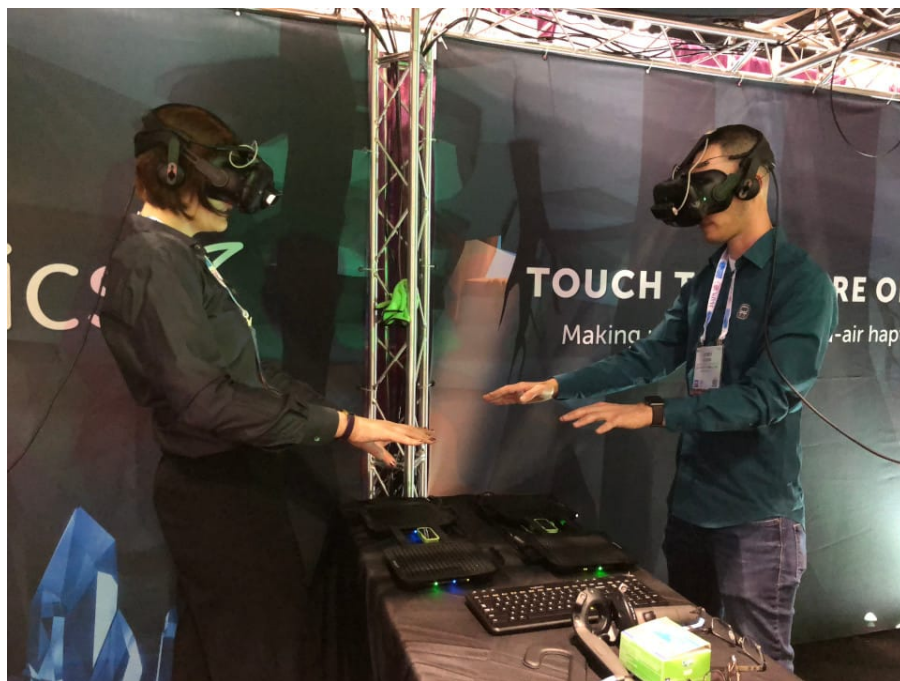
Figure 9: STRATOS Explore haptic device used by two users in VR. The haptic device is capable of delivering tactile experiences to the users. Image source: https://www.ultraleap.com/product/stratos-explore/
